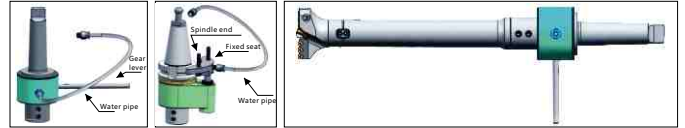
Installation diagram of Morse handle Schematic diagram of BT handle installation
